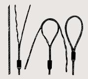
In the standard flemish eye mechanical splice, wire rope is separated into two parts: three adjacent strands to one part and three adjacent strands along with the core to the other part. The two parts are then re-laid back in opposite directions to form an eye and ends are secured with a pressed metal sleeve.
